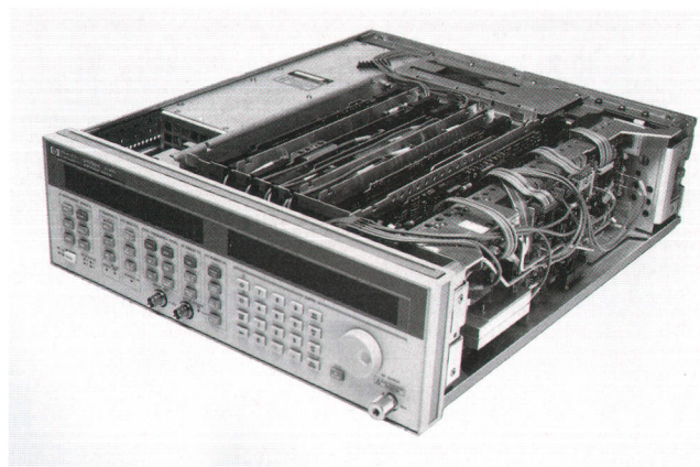
Fig. 8. Internal view of the HP 83750 chassis.
