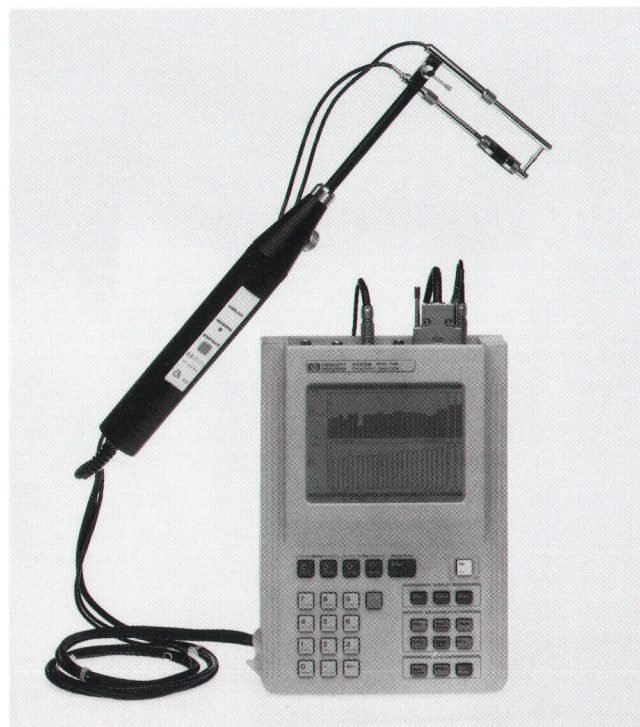
Fig. 1. The HP 3569A real-time frequency analyzer and the HP 35230A sound intensity probe.
