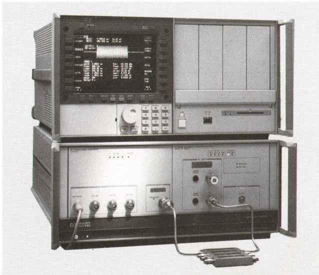
Fig. 3. An example of a modular measurement system consisting of an HP 70340A signal generator (highlighted) and an HP 71500A microwave transition analyzer.
